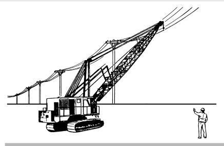
Use a signaller if equipment or its load is closer than one boom length to overhead powerlines.
